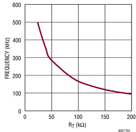
Figure 1. Timing Resistor ( $R_T$ ) Value
